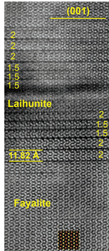
FIGURE 5. A [100]-zone-axis Z-contrast image showing interface between fayalite and laihunite domains with doubled (2) and tripled (1.5) periodicities along the c -axis.
